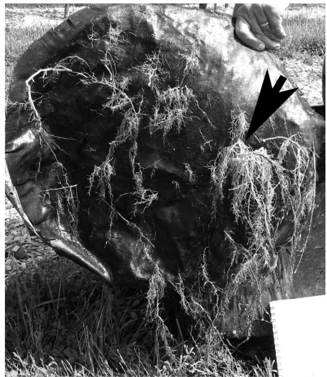
Fig. 4. Root penetration through woven geotextile. Roots of green ash emerge through woven geotextile where compacted subsoil has been washed away. Arrow indicates point of root proliferation where geotextile fiber is ruptured. (Exp. 2).
