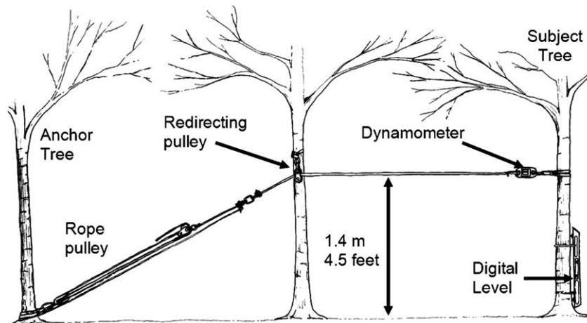
**Fig. 1.** Schematic drawing of the rigging system used to apply and measure force required to deflect the trunks of experimental (subject) trees growing in the engineered soil mixes. In the drawing, the proximity of the anchor, redirect, and subject trees is not drawn to scale. For subject trees at the end of planting rows, the winch system was anchored to a tow hook on the bumper of a vehicle positioned in the same manner as an anchor tree.
